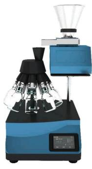
The sample divider SD110 is used to evenly divide a whole sample into 6, 8, 10 evenly small samples. Each sample has the same physical and chemical properties, and can represent the properties of the whole sample, and the sample separator is currently a more accurate sample separator on the market.
